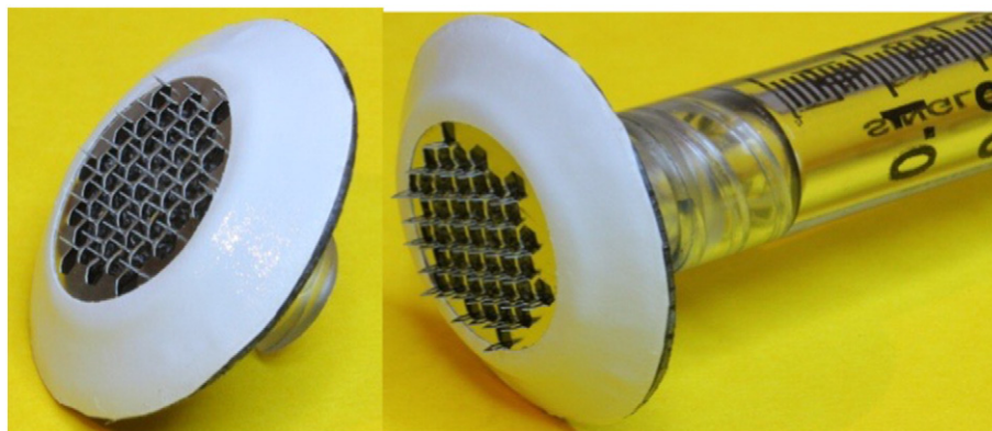
Fig. 1. AdminPen™ device comprised of an array of 43 metallic microneedles of 1100 nm length in 1 cm sq area of circular microneedle array made of SS316 stainless steel, attached to a syringe (Image produced with a permission from AdminMed/nanoBioSciences LLC).
