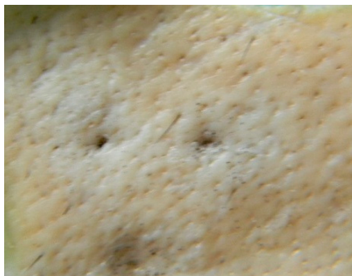
Figure 14. Porcine skin pierced with FSBP (left) and NC (right) single microneedle.
