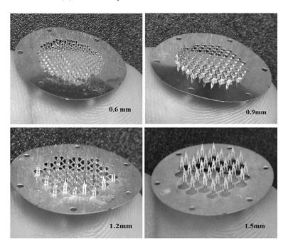
Fig. (2). Adminpatch<sup>®</sup> microneedle arrays used in the study.
