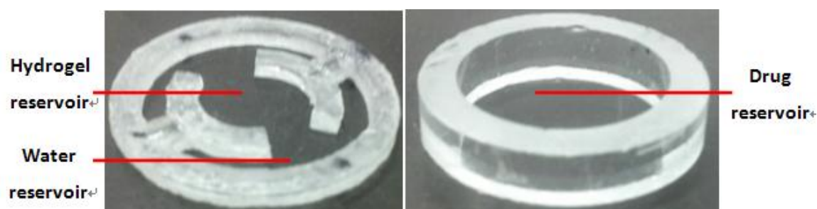
Figure 2.10. Transparent substrate for hydrogel swelling characterization.
